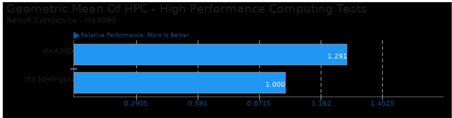
Geometric mean based upon tests: pts/rodinia, pts/arrayfire, pts/gromacs, pts/ncnn, pts/caffe, pts/shoc, pts/plaidml and pts/lczero
