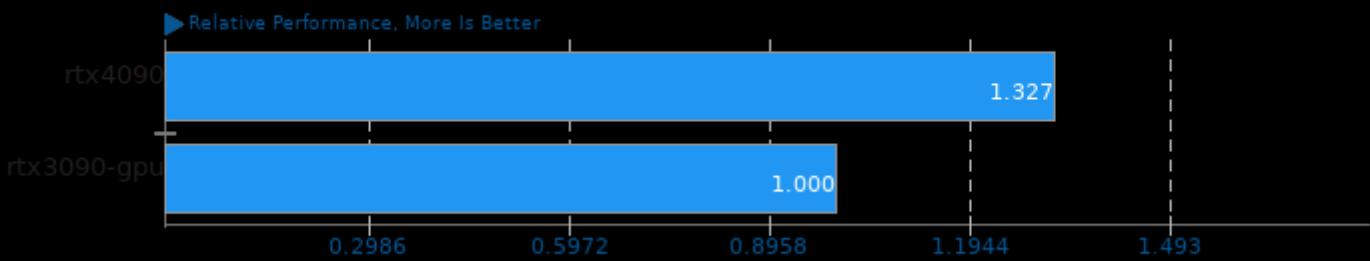
Geometric mean based upon tests: pts/vkfft, pts/vkresample, pts/vkpeak, pts/ncnn, pts/realsr-ncnn, pts/waifu2x-ncnn, pts/betsy and pts/libplacebo
