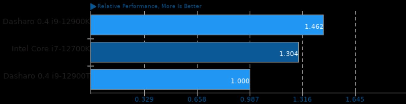
Geometric mean based upon tests: pts/x264, pts/x265, pts/compress-7zip, pts/build-linux-kernel, pts/openssl, system/gimp, pts/pybench and pts/phpbench
