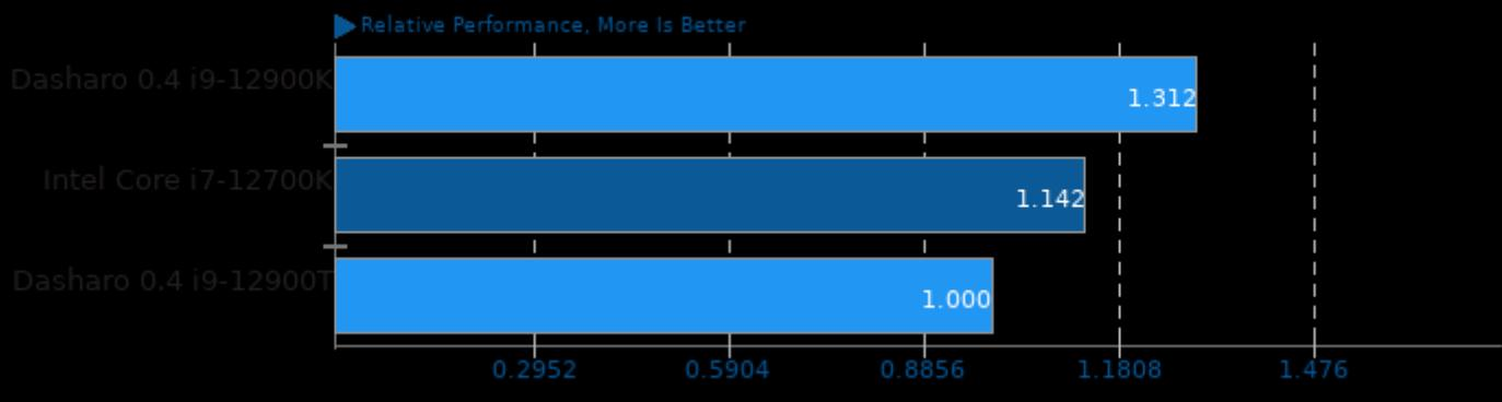
Geometric mean based upon tests: pts/x264, pts/x265, pts/ffmpeg, pts/encode-mp3, pts/encode-flac, system/gimp, system/rsvg and system/gegl
