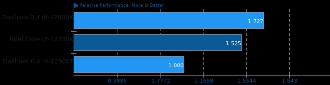
Geometric mean based upon tests: pts/x264, pts/x265, pts/ffmpeg, pts/compress-7zip, pts/build-linux-kernel and pts/build-nodejs
