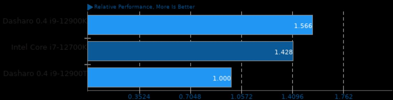
Geometric mean based upon tests: pts/build-linux-kernel, pts/compress-7zip, pts/x264, pts/x265, pts/encode-flac, pts/encode-mp3, pts/openssl, pts/phpbench, system/cryptsetup and system/octave-benchmark
