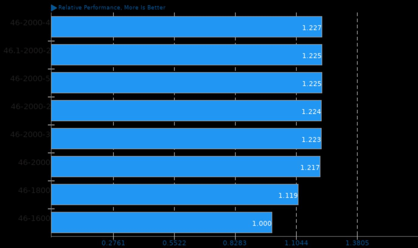
Geometric mean based upon tests: pts/ramspeed, pts/stream, pts/t-test1, pts/cachebench, pts/tinymembench and pts/mbw
