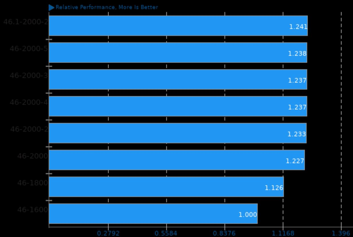
Geometric mean based upon tests: pts/ramspeed and pts/stream
