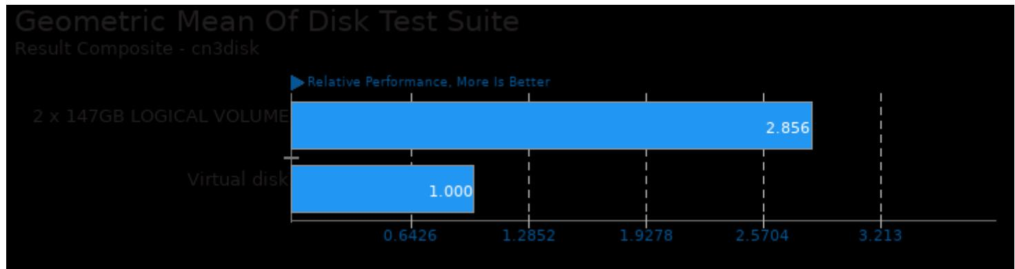
Geometric mean based upon tests: pts/sqlite, pts/fs-mark, pts/dbench and pts/fio
