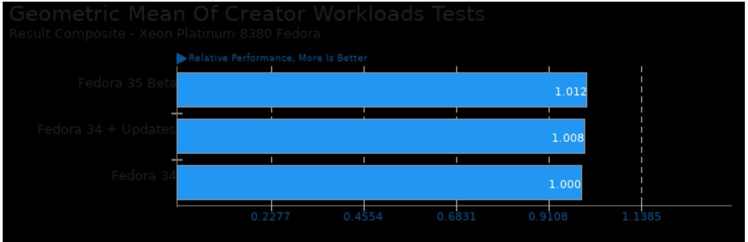
Geometric mean based upon tests: pts/ospray, pts/blender, pts/appleseed, pts/v-ray, pts/svt-vp9, pts/svt-hevc, pts/x265, pts/svt-av1, pts/jpegxl, pts/embree, pts/oidn, pts/opencv, pts/build-godot and pts/synthmark
