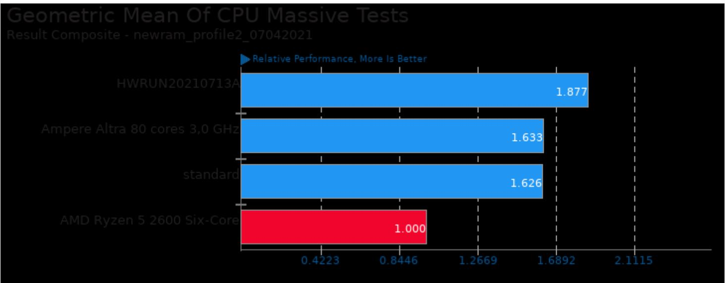
Geometric mean based upon tests: pts/cachebench, pts/mbw, pts/ramspeed, pts/stream, pts/t-test1 and pts/tinymembench
