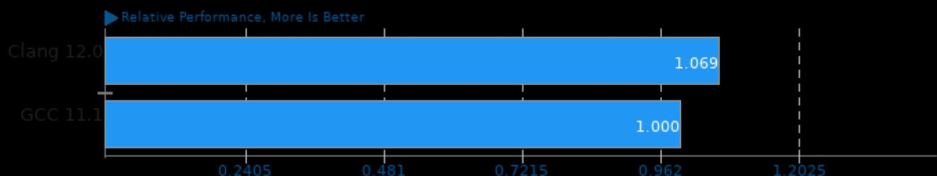
Geometric mean based upon tests: pts/c-ray, pts/coremark, pts/svt-vp9, pts/svt-hevc, pts/x265, pts/kvazaar, pts/svt-av1, pts/primesieve, pts/graphics-magick, pts/onednn, pts/compress-zstd, pts/aobench and pts/pgbench
