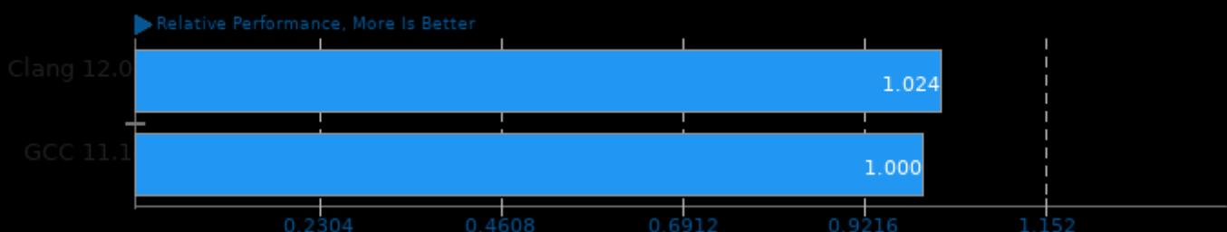
Geometric mean based upon tests: pts/svt-vp9, pts/svt-hevc, pts/x265, pts/kvazaar and pts/svt-av1
