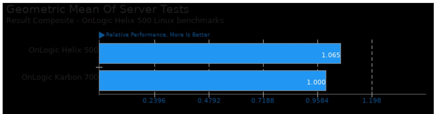
Geometric mean based upon tests: pts/simdjson, pts/sqlite-speedtest, pts/leveldb and pts/influxdb
