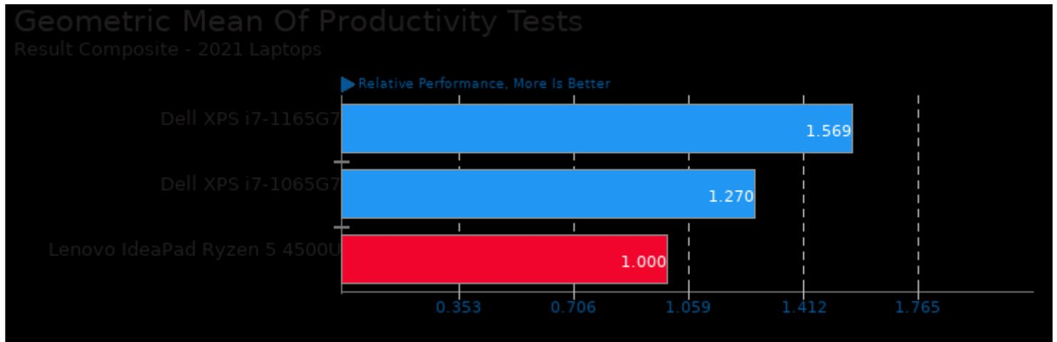
Geometric mean based upon tests: system/libreoffice and system/rsvg
