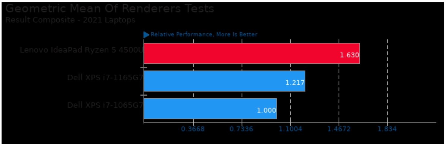
Geometric mean based upon tests: pts/yafaray, pts/blender, pts/appleseed, pts/luxcorerender and pts/indigobench
