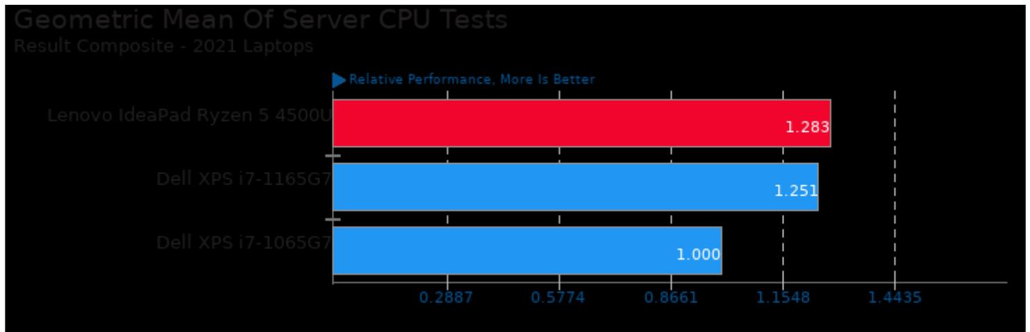
Geometric mean based upon tests: pts/svt-av1, pts/svt-vp9, pts/x265, pts/dav1d, pts/stockfish, pts/build-linux-kernel, pts/compress-zstd, pts/tjbench, pts/blender, pts/appleseed and pts/pybench
