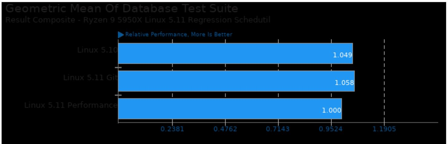
Geometric mean based upon tests: pts/sqlite-speedtest, pts/keydb, pts/rocksdb, pts/pgbench, pts/couchdb and pts/influxdb
