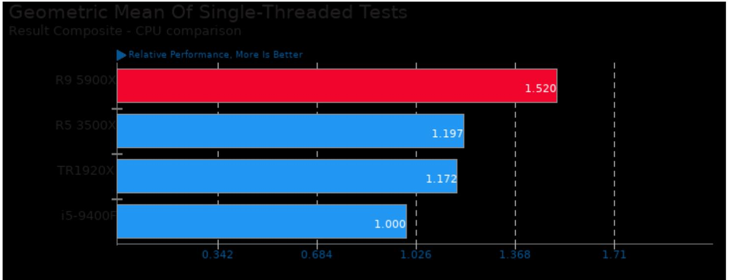
Geometric mean based upon tests: pts/lzbench and pts/botan
