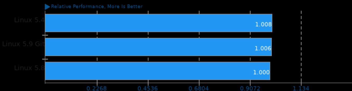
Geometric mean based upon tests: pts/build-apache, pts/build-llvm, pts/build-linux-kernel, pts/compress-xz, pts/compress-zstd, pts/crafty, pts/dolby, pts/hint, pts/hmmer, pts/lammps, pts/lczero, pts/mafft, pts/onnednn, pts/namd, pts/rodinia, pts/blender and system/tesseract-ocr
