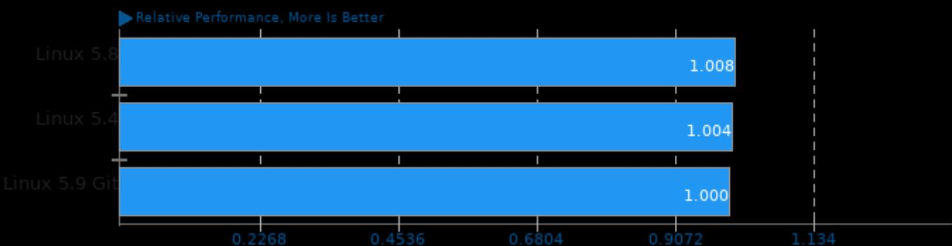
Geometric mean based upon tests: pts/build-apache, pts/build-linux-kernel, pts/build-gdb and pts/build-llvm
