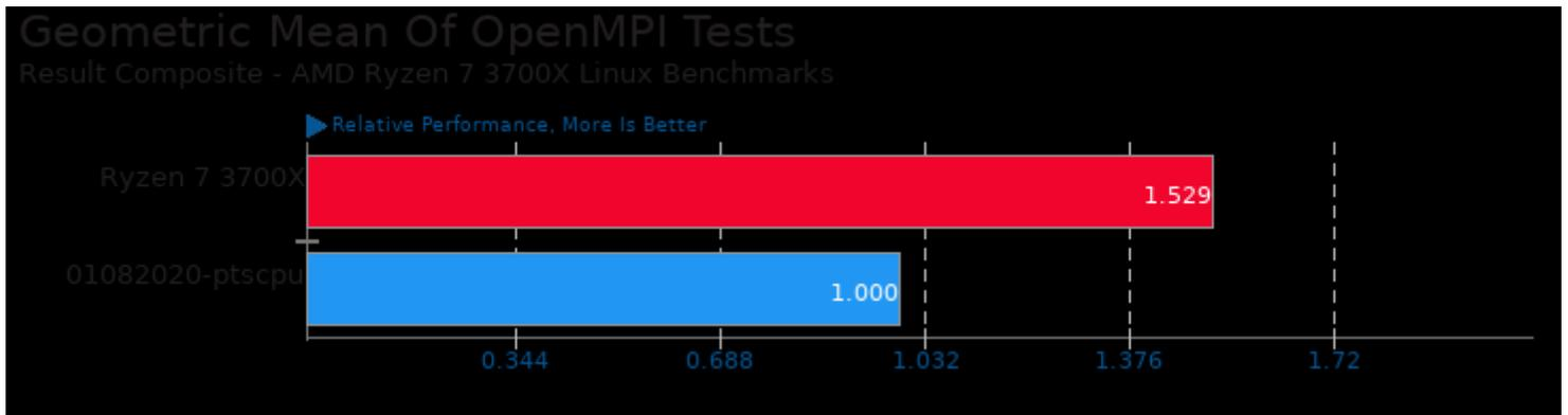
Geometric mean based upon tests: pts/npb, pts/hpcc, pts/parboil, pts/cloverleaf, pts/rodinia, pts/clomp and pts/nero2d
