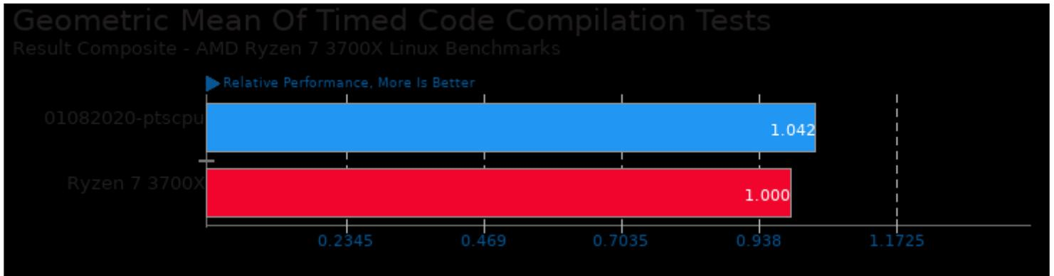
Geometric mean based upon tests: pts/build-php, pts/build-linux-kernel, pts/build-gcc and pts/build-llvm
