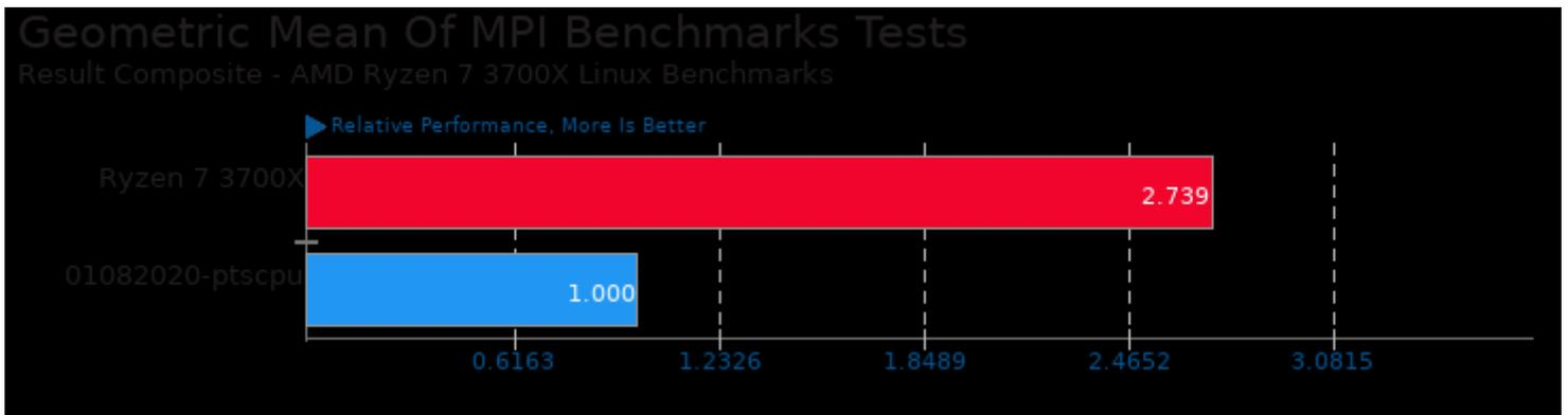
Geometric mean based upon tests: pts/hpcc, pts/nero2d, pts/hpcg, pts/mrbayes and pts/npb
