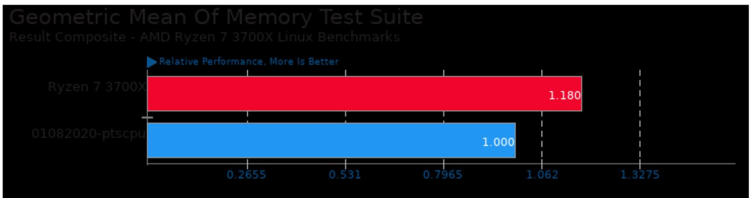
Geometric mean based upon tests: pts/ramspeed, pts/stream, pts/t-test1, pts/cachebench, pts/tinymembench and pts/mbw
