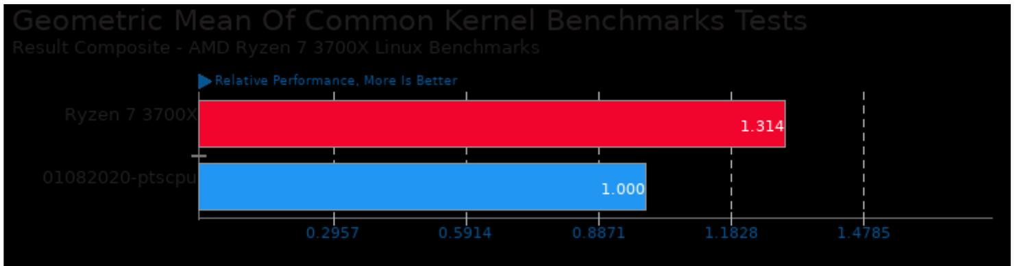
Geometric mean based upon tests: pts/apache, pts/pgbench, pts/tinymembench, pts/mbw, pts/t-test1, pts/openssl, pts/ctx-clock, pts/hackbench and pts/stress-ng
