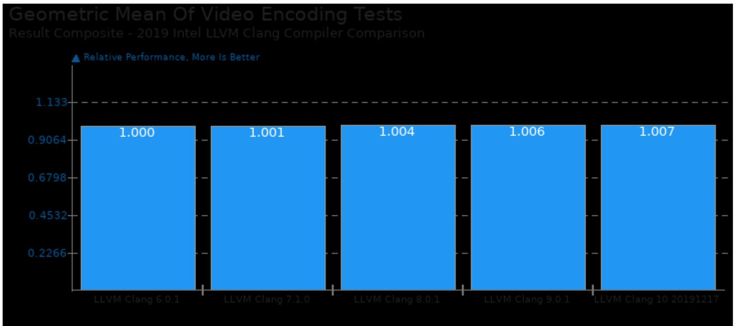
Geometric mean based upon tests: pts/svt-vp9, pts/svt-hevc, pts/x264, pts/x265, pts/vpxenc, pts/dav1d, pts/svt-av1 and pts/libgav1
