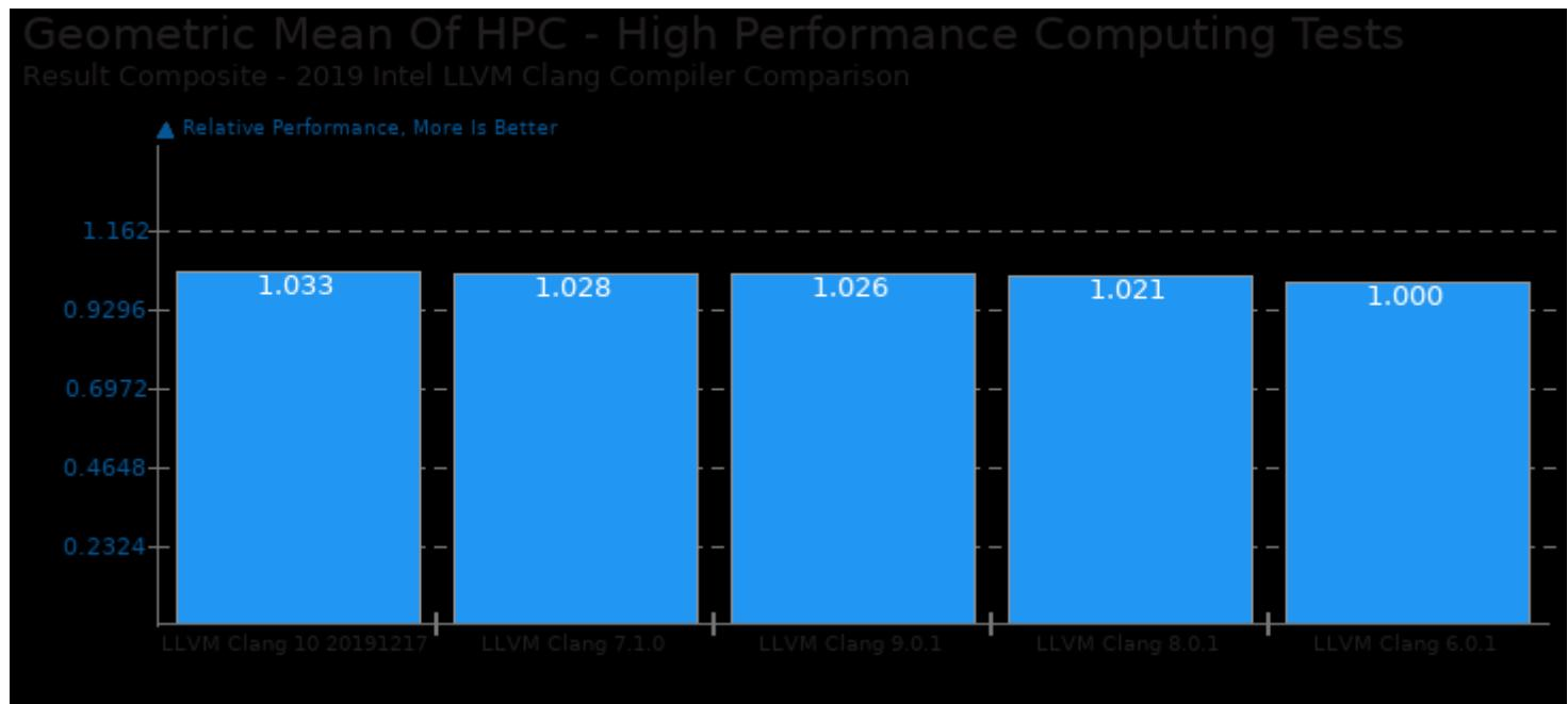
Geometric mean based upon tests: pts/himeno, pts/mrbayes and pts/hmmer
