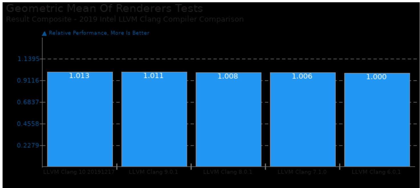
Geometric mean based upon tests: pts/c-ray, pts/tungsten and pts/aobench
