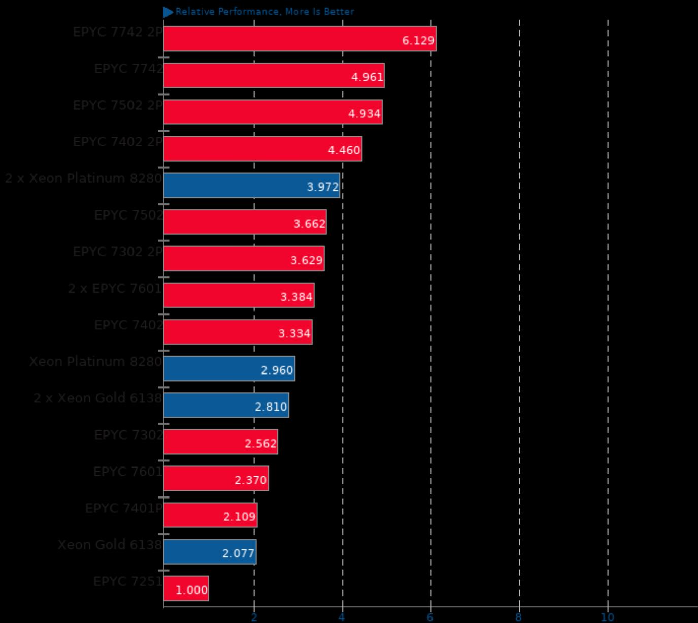
Geometric mean based upon tests: pts/vpxenc, pts/stockfish, pts/build-llvm, pts/c-ray, pts/compress-7zip, pts/john-the-ripper, pts/dav1d, pts/x264, pts/x265, pts/tungsten, pts/aom-av1, pts/svt-av1 and pts/svt-vp9
