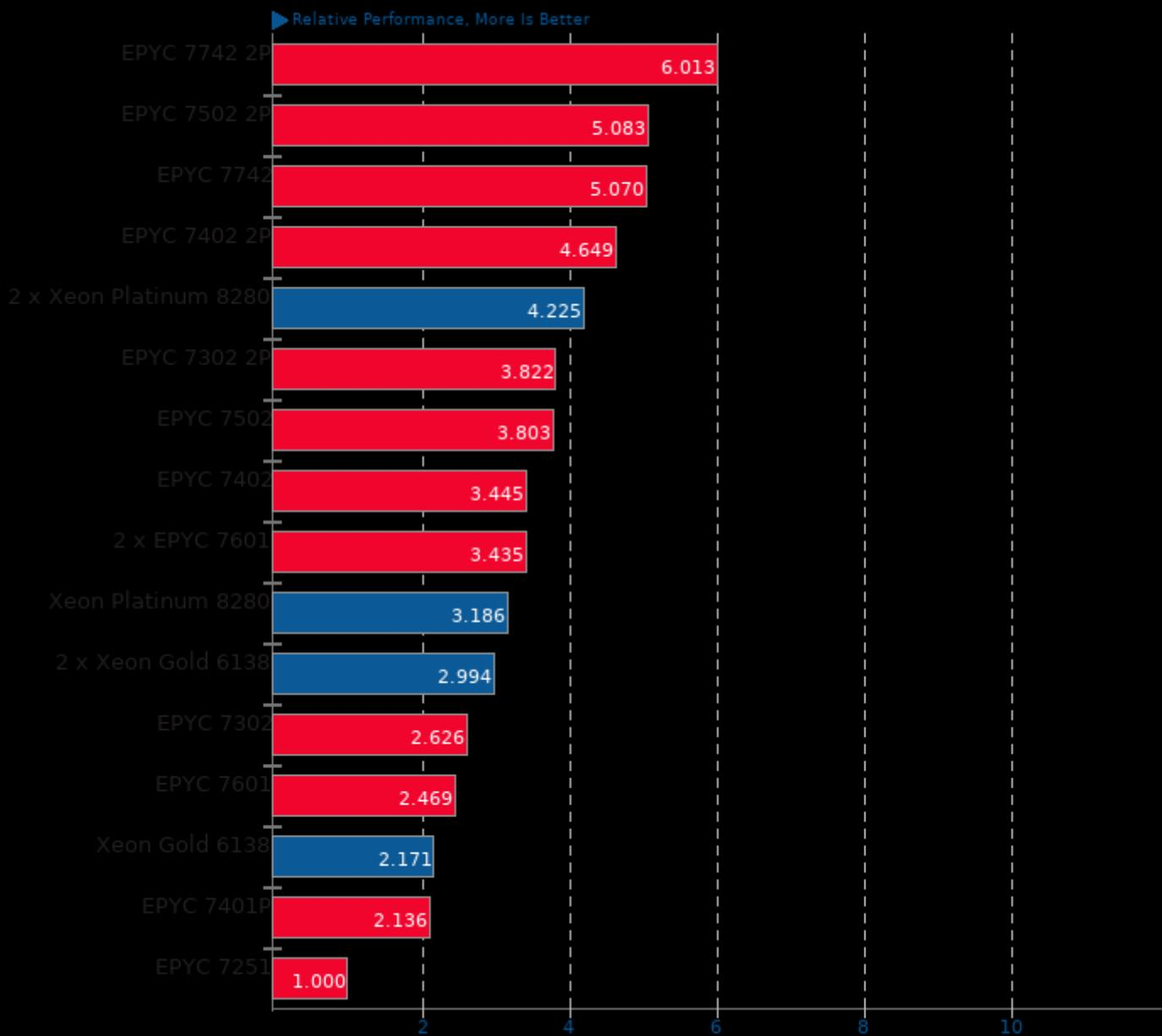
Geometric mean based upon tests: pts/c-ray, pts/povray, pts/blender, pts/tungsten, pts/appleseed, pts/svt-vp9, pts/svt-hevc, pts/x264, pts/x265, pts/vpxenc, pts/dav1d, pts/aom-av1, pts/svt-av1 and pts/neatbench
