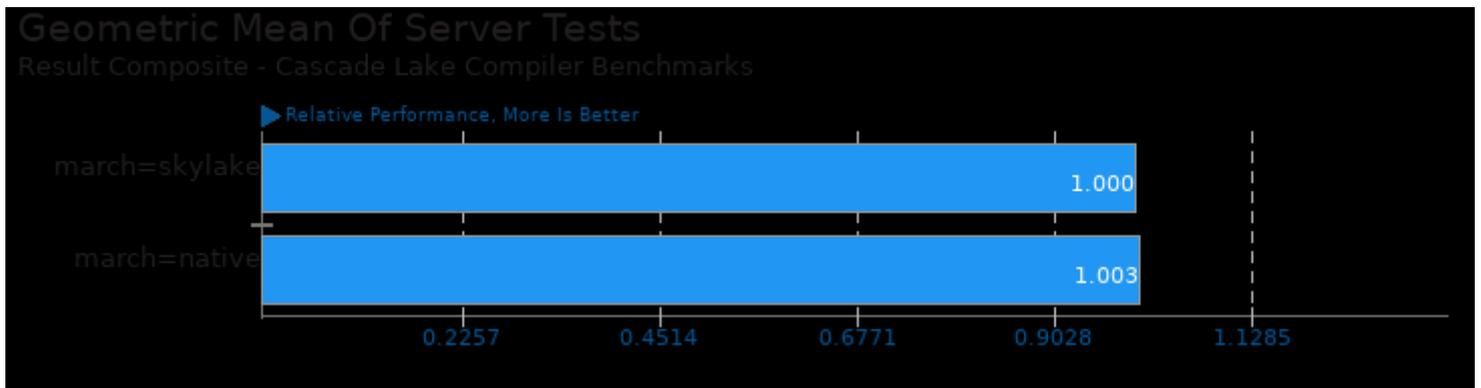
Geometric mean based upon tests: pts/apache, pts/nginx, pts/apache-siege, pts/pgbench, pts/mcperft and pts/openssl
