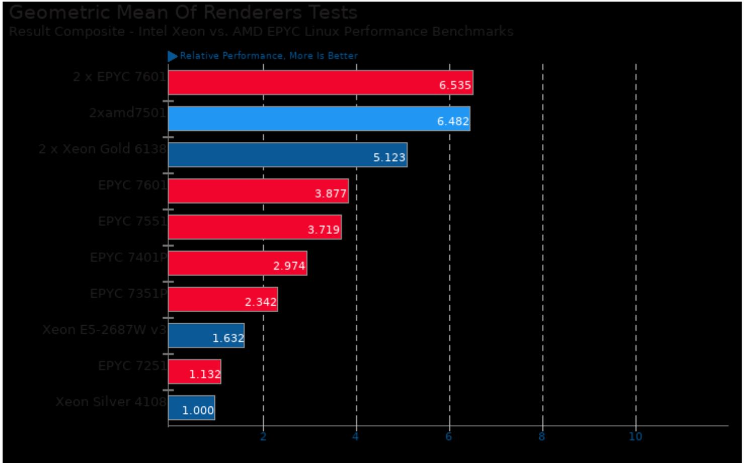
Geometric mean based upon tests: pts/tachyon, pts/povray, pts/blender and pts/v-ray
