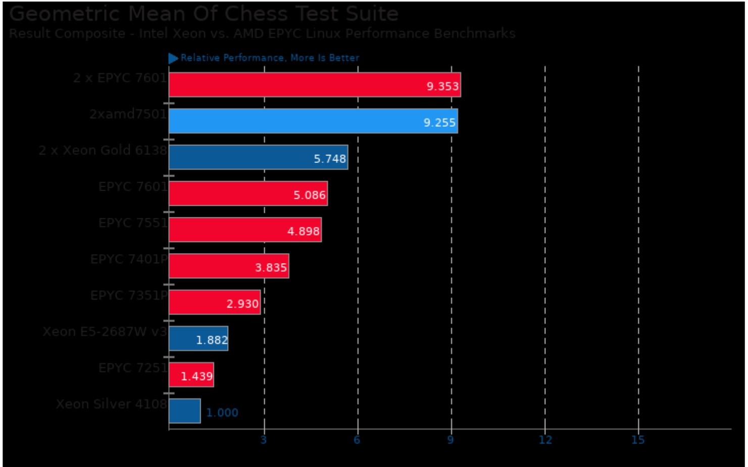
Geometric mean based upon tests: pts/stockfish, pts/asmfish and pts/m-queens
