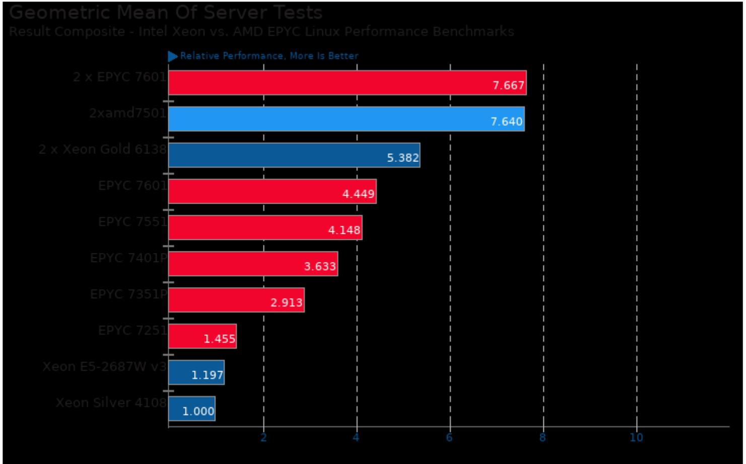
Geometric mean based upon tests: pts/ebizzy and pts/openssl
