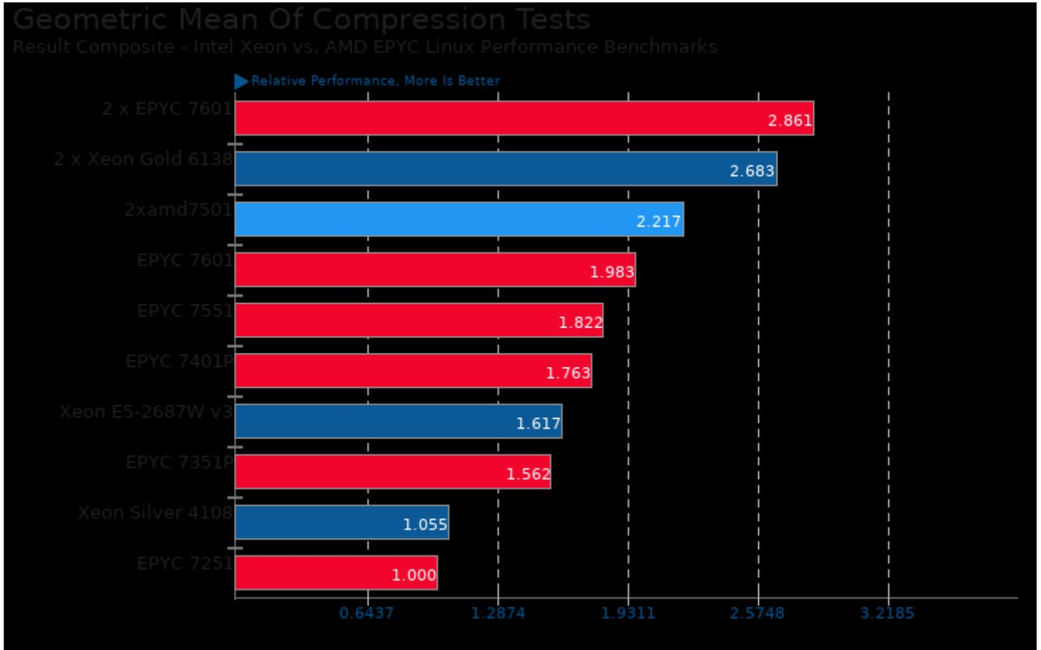
Geometric mean based upon tests: pts/compress-7zip and pts/compress-rar
