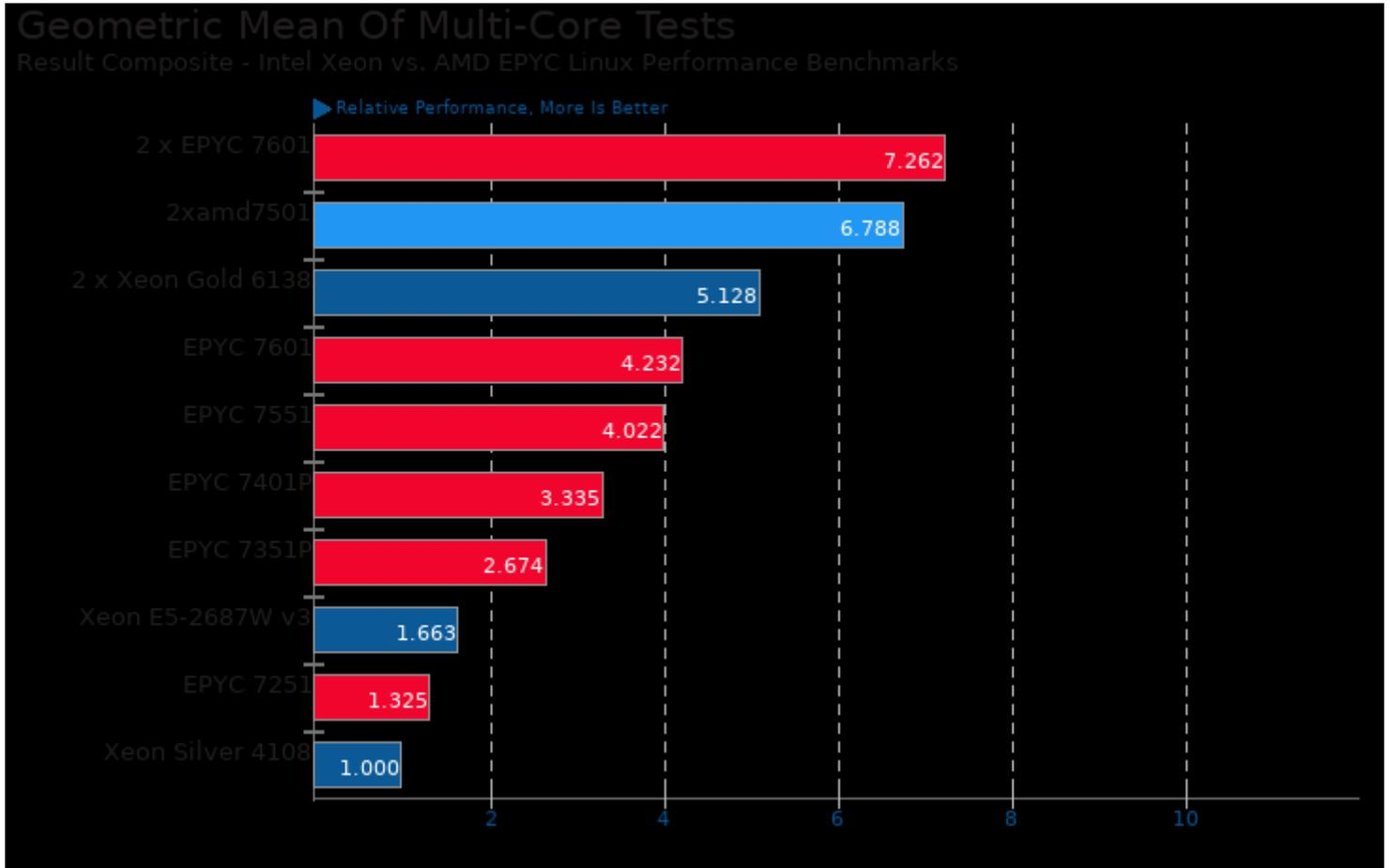
Geometric mean based upon tests: pts/blender, pts/sysbench, pts/tachyon, pts/povray, pts/stockfish, pts/m-queens, pts/primesieve, pts/john-the-ripper, pts/namd, pts/asmfish, pts/ebizzy, pts/compress-7zip, pts/build-linux-kernel, pts/build-llvm and pts/v-ray
