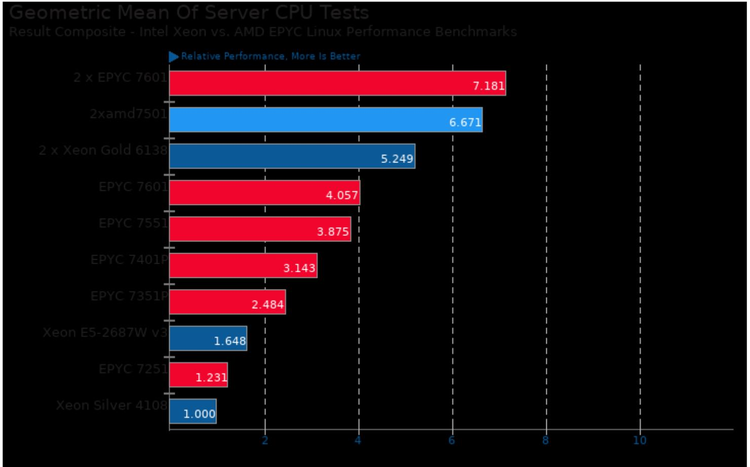
Geometric mean based upon tests: pts/namd, pts/john-the-ripper, pts/compress-7zip, pts/stockfish, pts/asmfish, pts/build-linux-kernel, pts/build-llvm, pts/povray, pts/m-queens, pts/openssl, pts/sysbench and pts/blender
