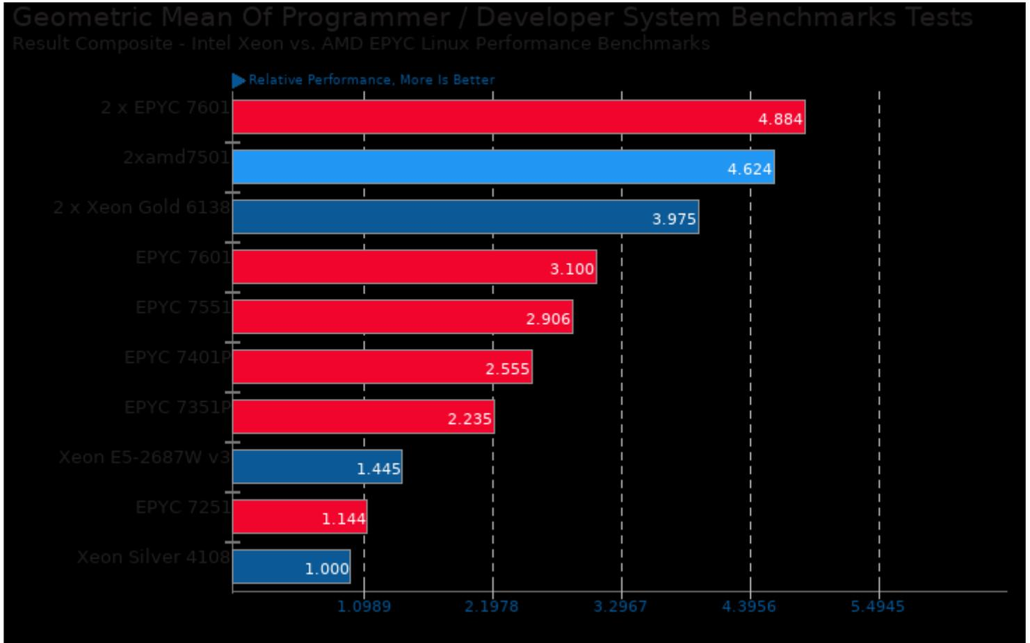
Geometric mean based upon tests: pts/build-linux-kernel and pts/build-llvm
