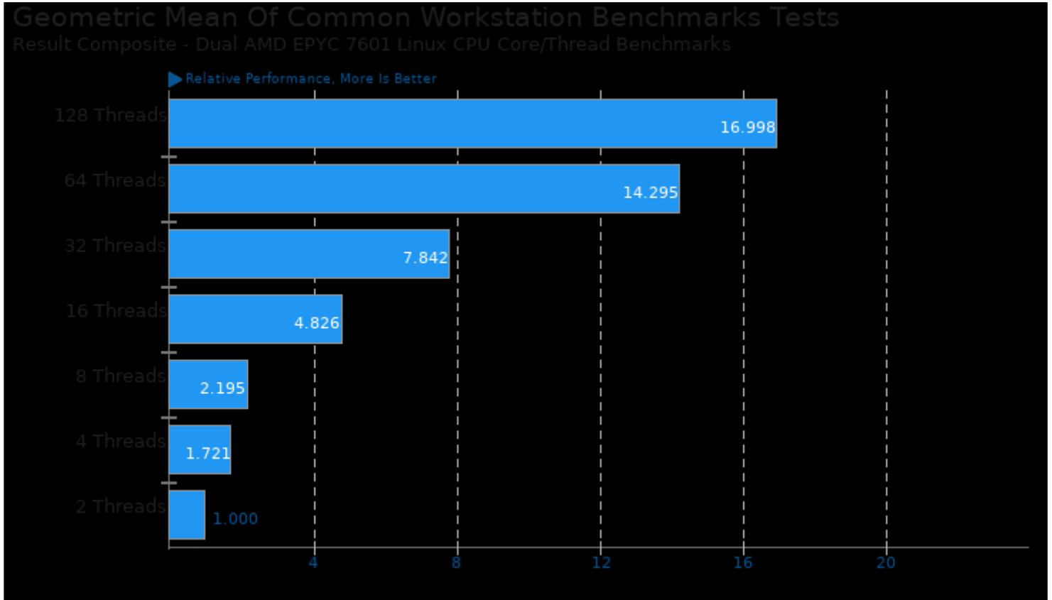
Geometric mean based upon tests: pts/rodinia, pts/himeno and pts/brl-cad
