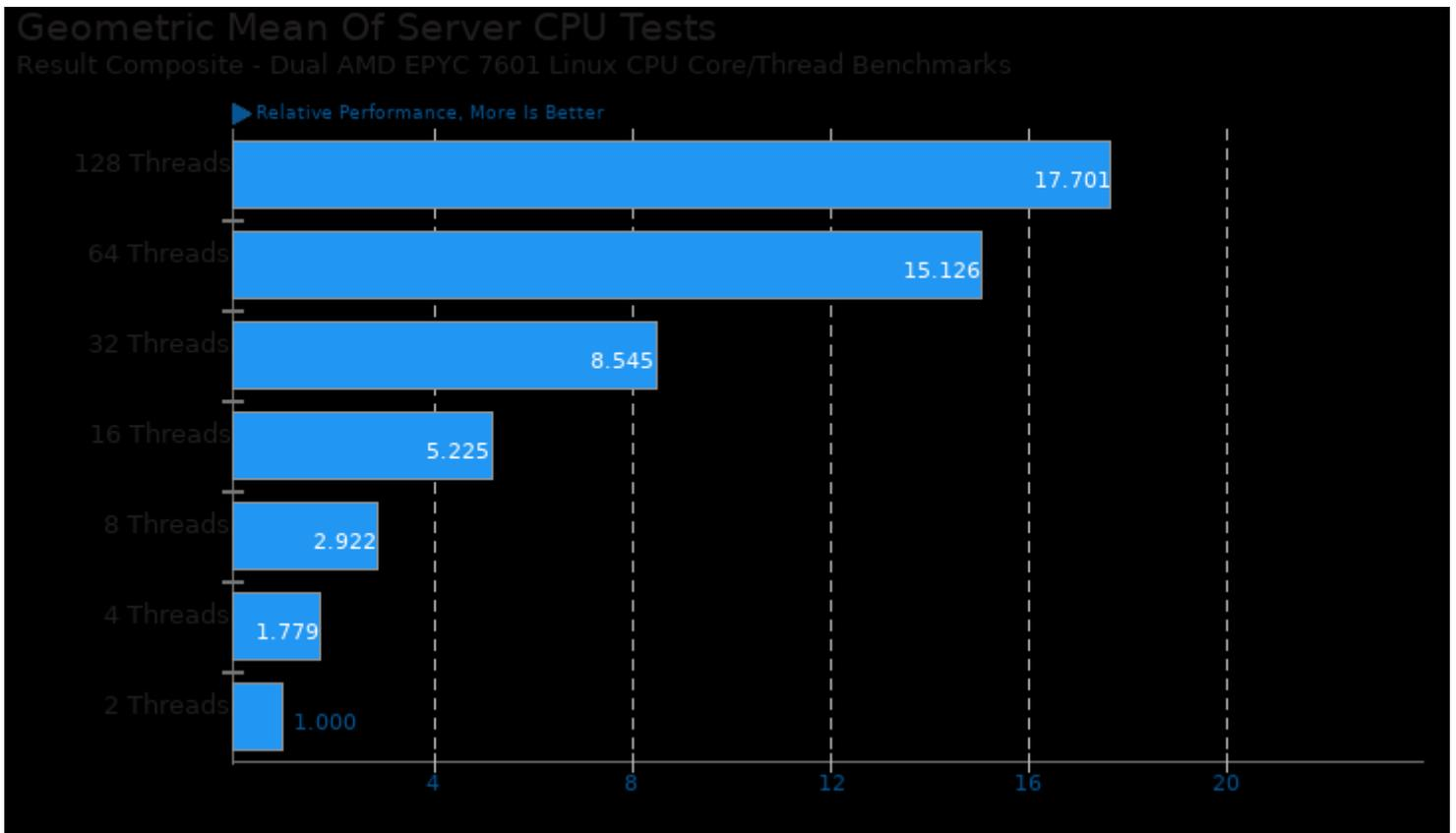
Geometric mean based upon tests: pts/rodinia, pts/namd, pts/dacapobench, pts/x264, pts/himeno, pts/compress-7zip, pts/stockfish, pts/asmfish, pts/build-linux-kernel, pts/build-llvm, pts/c-ray, pts/povray, pts/rust-mandel, pts/m-queens,
